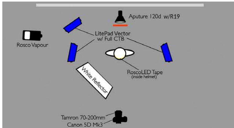
It's worth noting that Jay P. used several other Rosco products in his shot. He had three of our LitePad Vector CCT LED lights with Full CTB Cinegel filters positioned just out of frame on either side of the model to add a cool-colored rim light. He also added a piece of Roscolux #19 Fire on the backlight, along with some hazy fog from his Vapour Fog Machine to add in a reddish haze.
