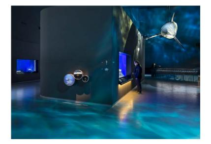
Kongshaug and his team installed over forty Rosco DMX-controlled X24 Effect Projectors throughout the building's 53 aquariums, giving Kongshaug complete control of the speed, direction and coverage of the projected water effects being created.
