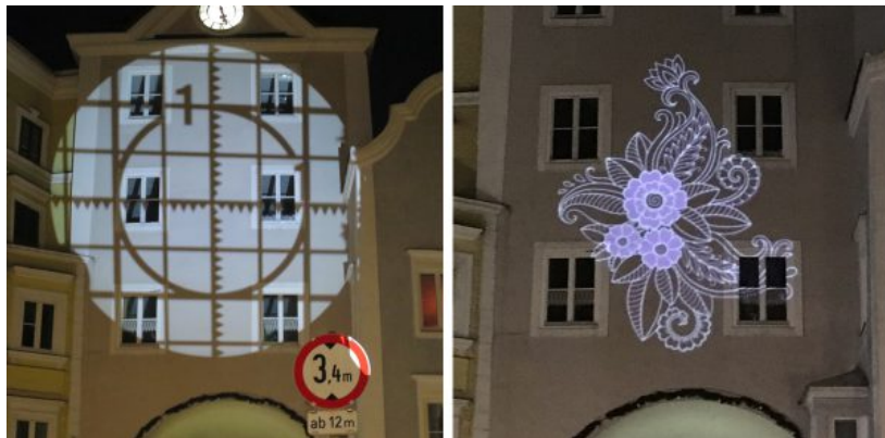
R77888 Line Up Grid projected (L) and the resulting Custom Gobo perfectly projected (R)
