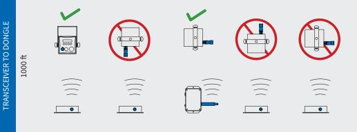
Antenna positions for the sending Transceiver and the corresponding receiving Dongle, Fixture Antenna or Transceiver can significantly affect signal quality. For optimum performance reference the sending and receiving pairings and positions in the diagrams to the left.
